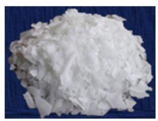
**GH360WAX** is a polyethylene wax. It is insoluble or at most, very sparingly soluble in organic solvents at room temperature. It is soluble at elevated temperature in aliphatic, aromatic and chlorinated hydrocarbons and most other solvents which are not too polar.
